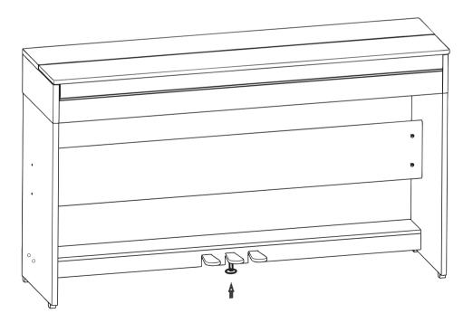
Attention: To avoid steeping on the pedal badly, the screw of footplatesupportshould contact with the ground closely after installation
